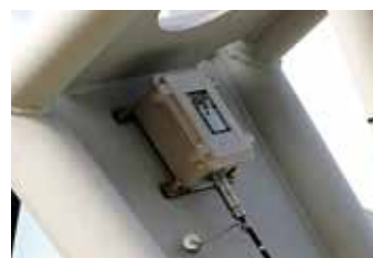
New boom angle sensor
