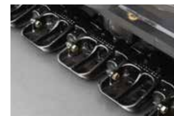
High-durability box type track shoes
